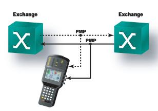
Long-term monitoring is simple with the SunSet E20c. Program a start and stop time, and the SunSet E20c takes care of the rest. The set may also be configured to print out every error or alarm condition, along with a date and timestamp. Histograms provide a graphical record of errors and alarms through time for easier correlation of repeating problems.
